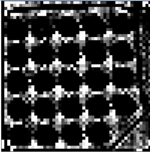
**Figure 5.7.** A reconstructed picture using measured data with a resolution of 50x50 pixels. The discriminator levels were set on  $0 \text{ mm}^{-1}$  and  $0.01 \text{ mm}^{-1}$ .
