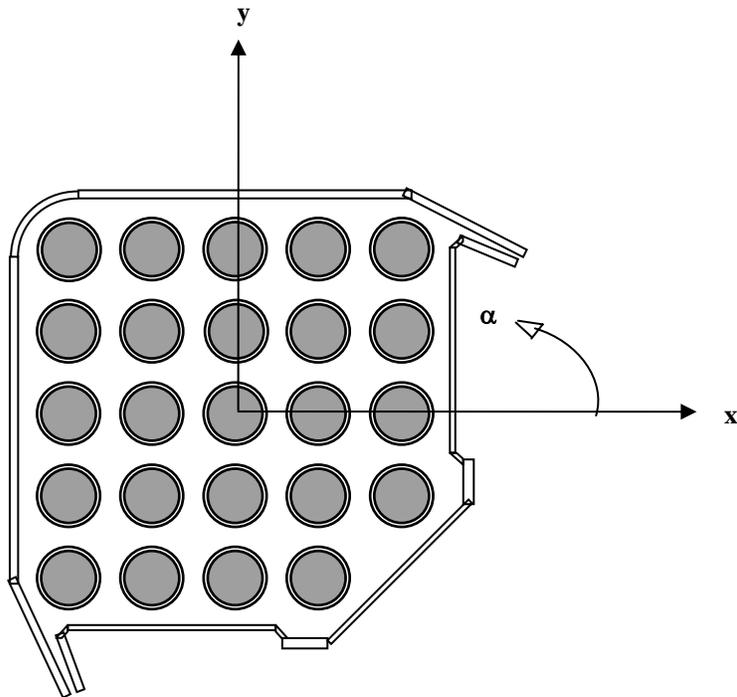
**Figure 5.9.** A schematic view of the coordinate system used when defining the fuel position of the fuel assembly tested in FRIGG.
