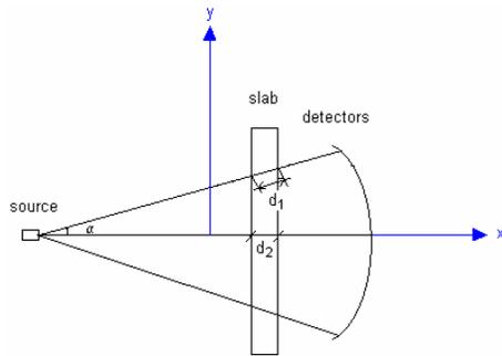
**Figure 4.4.** An illustration of the traveling distances of gamma-rays through a calibration slab.
