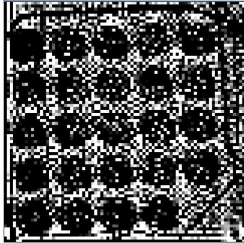
**Figure 5.8.** A reconstructed picture using measured data with a resolution of 80x80 pixels. The discriminator levels were set on  $0 \text{ mm}^{-1}$  and  $0.01 \text{ mm}^{-1}$ .
