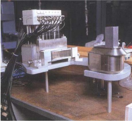
Figure 2.2. The FRIGG loop tomographic measuring table. Reproduced by courtesy of Westinghouse Electric Sweden AB.
