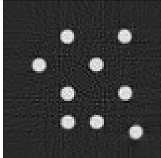
**Figure 5.14.** A reconstruction using simulated data where unique reference intensities for every measuring point were used. The resolution of the picture is 80x80 pixels. The grey-scale covers attenuation differences between  $-0.004 \text{ mm}^{-1}$  (white) and  $0.0006 \text{ mm}^{-1}$  (black).
