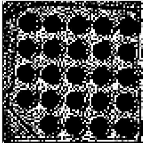
**Figure 5.11.** A reconstruction of measured data where the attenuation in the rods has been subtracted. The resolution is 80x80 pixels and the grey-scale level scheme goes from 0 to  $0.01 \text{ mm}^{-1}$ .
