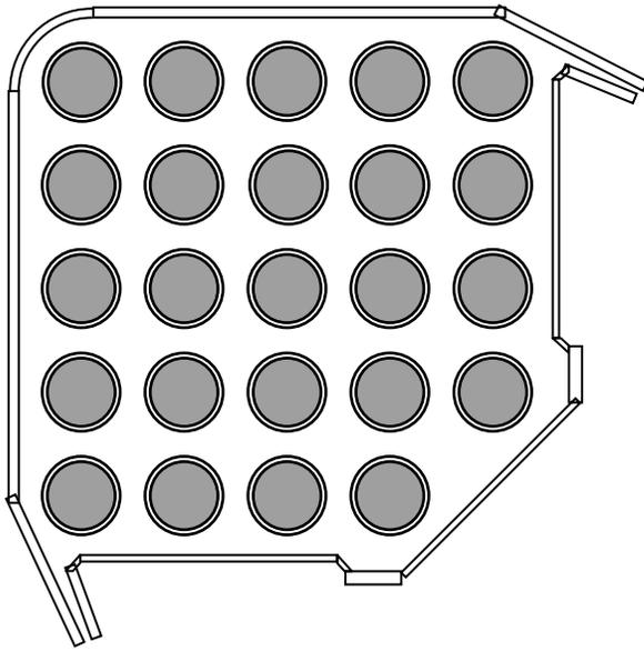
**Figure 4.2.** A schematic picture of a sub bundle that is being tested in FRIGG.
