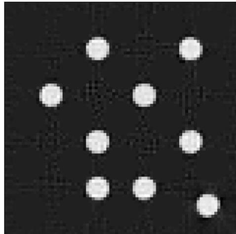
**Figure 5.16.** A reconstruction using simulated data and unique reference intensities for every data point. In this reconstruction, the difference in attenuation values of the rods was set to zero and such pixels were excluded in the reconstruction. The resolution of the picture is 80x80 pixels.
