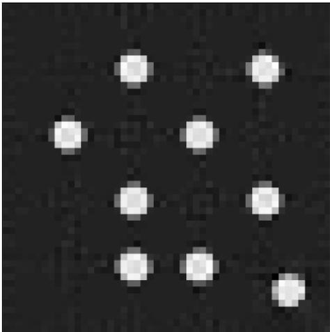
**Figure 5.15.** A reconstruction using simulated data and unique reference intensities for every data point. In this reconstruction, the difference in attenuation values of the rods was set to zero and such pixels were excluded in the reconstruction. The resolution of the picture is 50x50 pixels.
