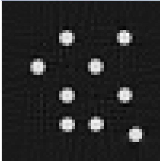
**Figure 5.13.** A reconstruction using simulated data where unique reference intensities for every measuring point were used. The resolution of the picture is 50x50 pixels. The grey-scale covers attenuation differences between  $-0.004 \text{ mm}^{-1}$  (white) and  $0.0006 \text{ mm}^{-1}$  (black).
