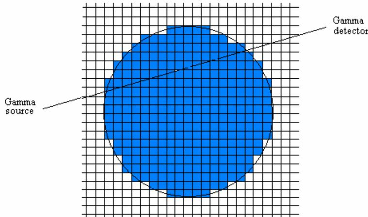
**Figure 3.1.** A principal sketch of quadratic pixel pattern covering one fuel rod.
