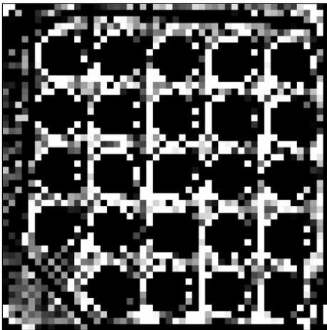
**Figure 5.10.** A reconstruction of measured data where the attenuation in the rods has been subtracted. The resolution is 50x50 pixels and the grey-scale level scheme goes from 0 to  $0.01 \text{ mm}^{-1}$ .
