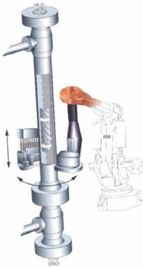
**Figure 2.1.** Positioning of the tomographic measuring equipment about the test loop FRIGG. Reproduced by courtesy of Westinghouse Electric Sweden AB.
