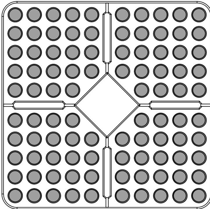
**Figure 1.1.** An axial cross section of a fuel assembly of type SVEA 96-S.
