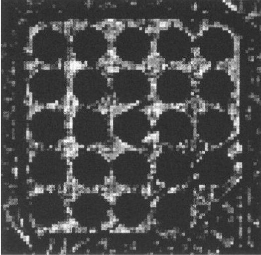
**Figure 2.5.** An example of a picture of the void distribution reconstructed by Westinghouse. Reprinted by courtesy of Westinghouse Electric Sweden AB.
