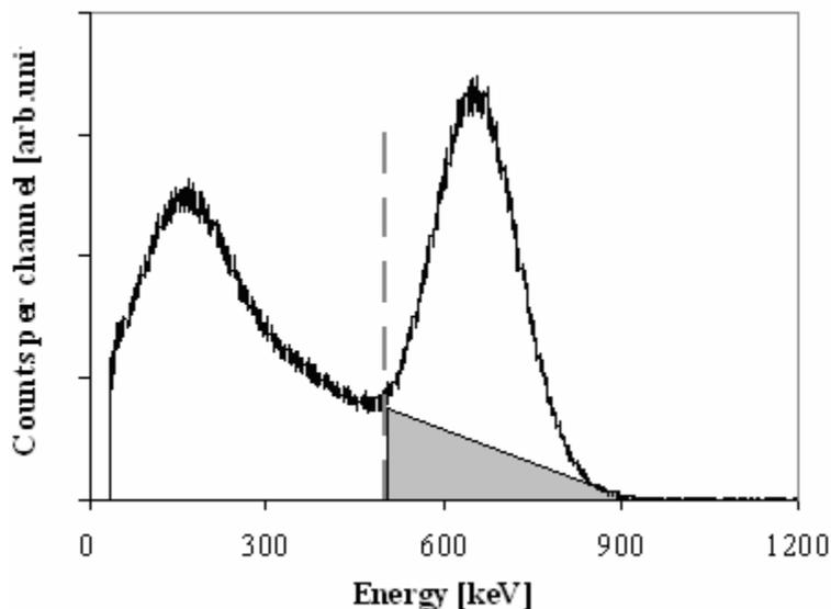
**Figure 2.4.** Gamma-ray spectrum of the 662 keV radiation from Cs-137 collected with a BGO detector. A possible setting of the lower discriminator level is also illustrated (from ref [3]). This type of data acquisition implies that the measured data will include background below the peak illustrated by a shaded triangle in the figure.
