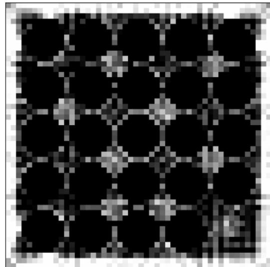
**Figure 5.2.** The result of a reconstruction of simulated data where the discriminator levels were set to  $0 \text{ mm}^{-1}$  (white) and  $0.01 \text{ mm}^{-1}$  (black). Here, it is possible to identify the nine regions with lower water density.
