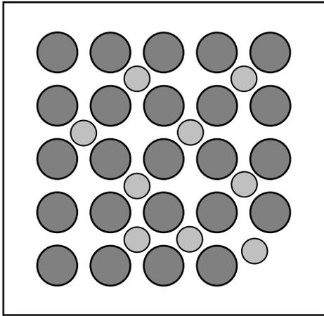
**Figure 4.1.** A schematic picture of the sub bundle used in the simulations. In the water surrounding the rods, nine cylinders with 60 % density were placed, simulating void.
