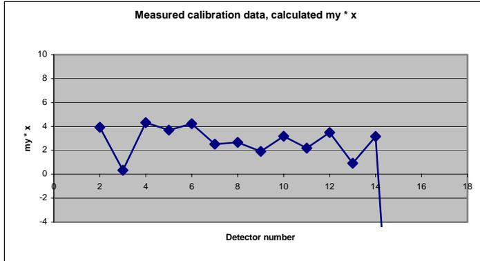
**Figure 4.8.** Plot of the calculated attenuation in slab, obtained in the analysis of calibration data.
