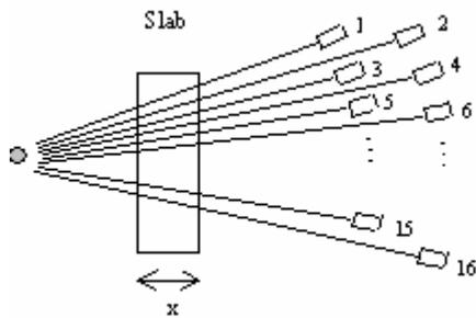
**Figure 4.5.** Gamma-ray distances through the slab at calibration.
