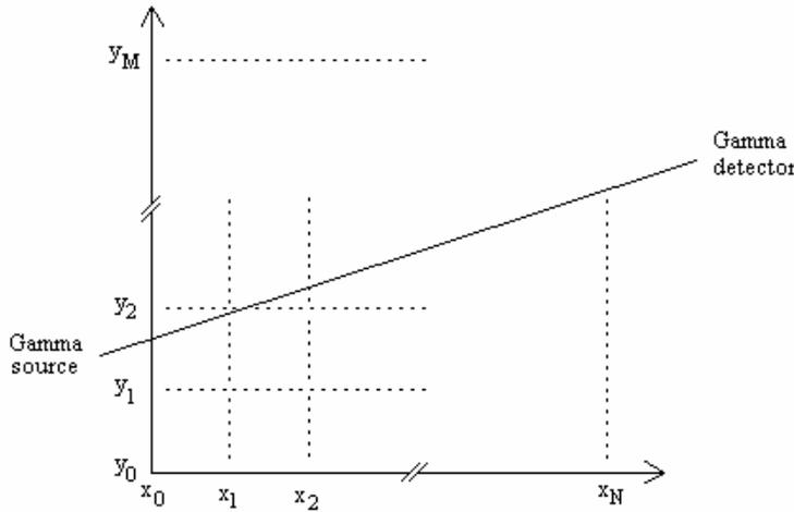
**Figure 3.2.** A schematic illustration of a coordinate system defining a quadratic pixel pattern.
