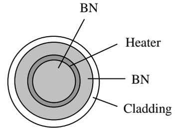
**Figure 4.3.** A cross section of a mockup rod used in FRIGG.
