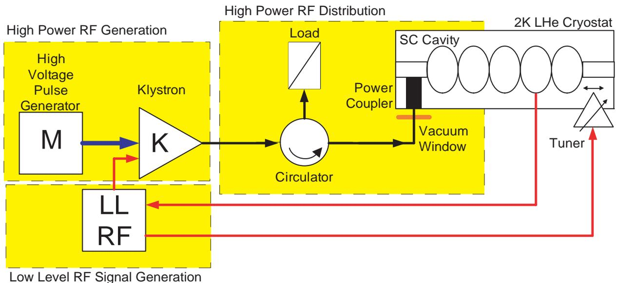
Figure 2: Basic layout of the RF system.
