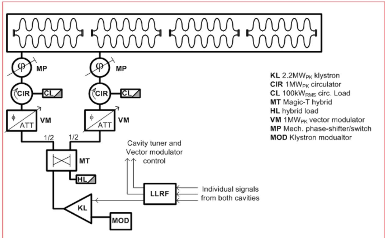
Figure 10: Layout of an RF distribution scheme where 1 klystron drives 2 cavities (courtesy D. Valuch) [8].
