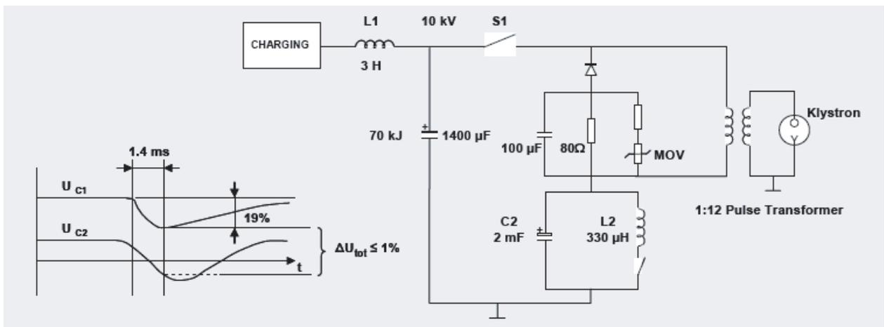
Figure 7: Topology of a klystron modulator (courtesy ILC) [7].
