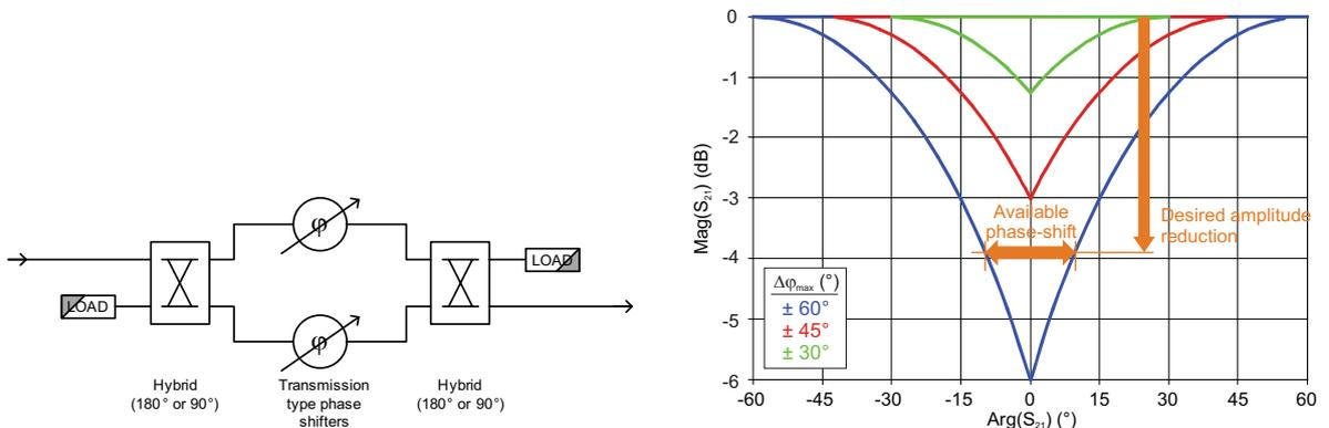
Figure 8: Schematic layout of a vector modulator (left) and its range of operation [8].
