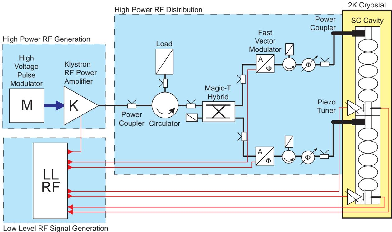
Figure 4: Configuration option of the RF test facility in which the two waveguide lines after the hybrid splitter are connected by vector modulators to superconducting cavities.
