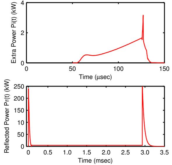
Figure 6: The extra incident power  $P_i(t)$  required to compensate the beam loading and the reflected power  $P_r(t)$  vs. time. Note that the time scales are different.
