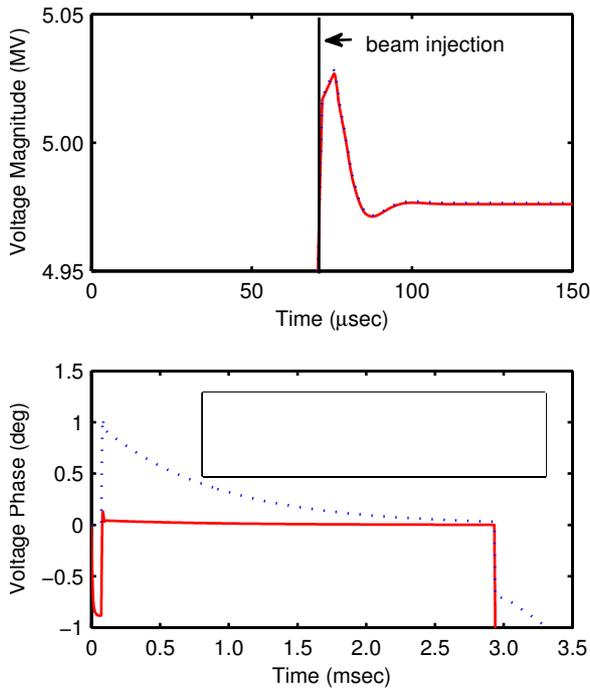
Figure 5: The voltage magnitude and phase of the controlled cavity with (red solid curve) and without (blue dotted curve) the cavity predetuning vs. time. Note that the time scales are different.
