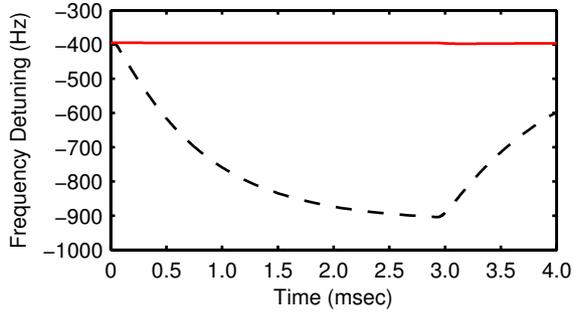
Figure 4: Dynamic detuning of the frequency caused by the electromagnetic pressure vs. time. The red solid curve and the black dashed curve stand for the cavity with and without control, respectively.
